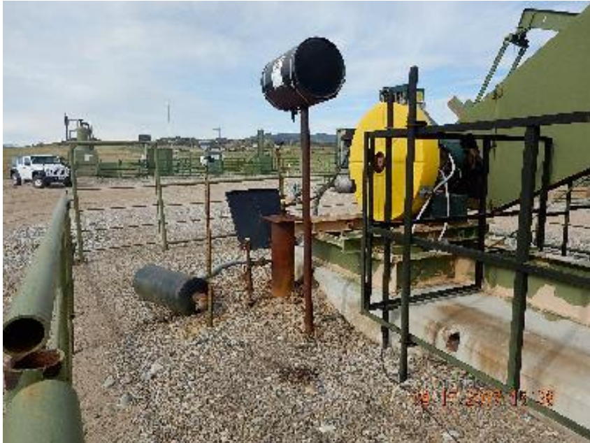
Photo 9: Lube oil tank with no spill prevention previous inspection.
