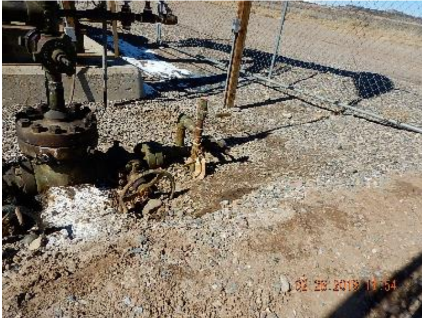
Photo 3: Impacted soil and unused 1" riser at the 15-2.
