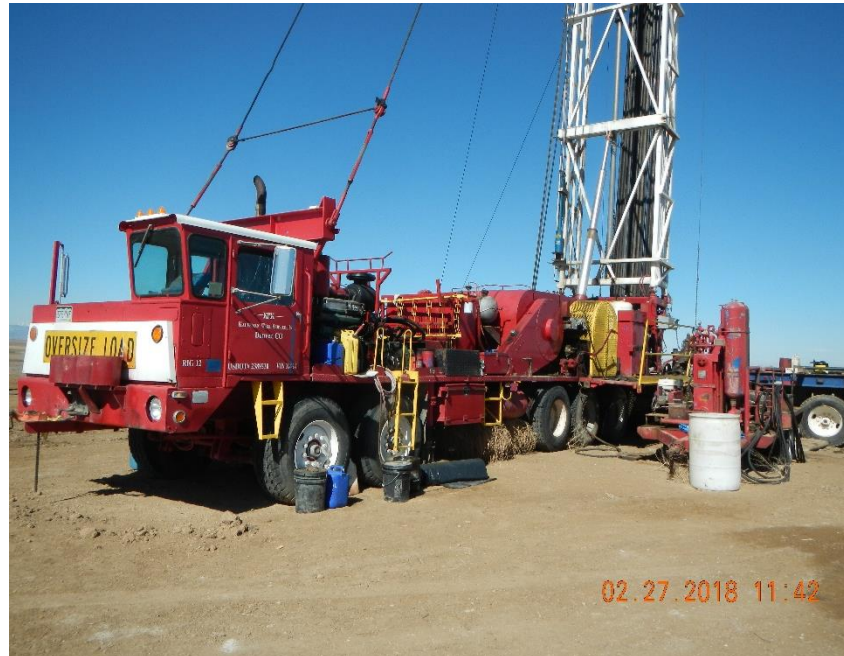
From SE view workover rig
