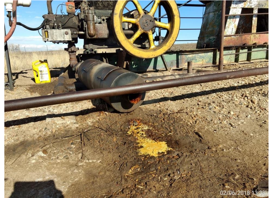
Prime Mover, Corrective Action: Stained soil around prime mover and exhaust.
