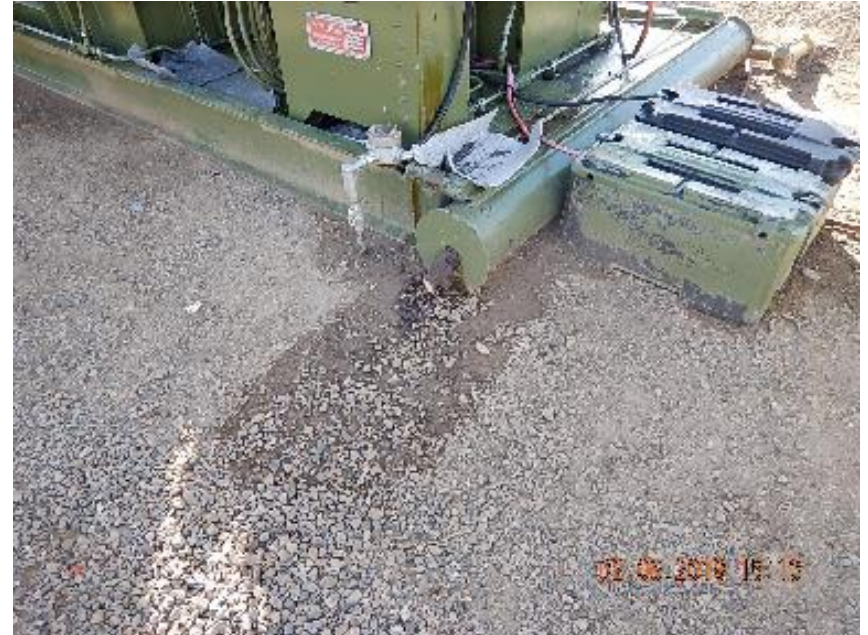
Photo 6: Impacted soil and gravel at compressor skid.
