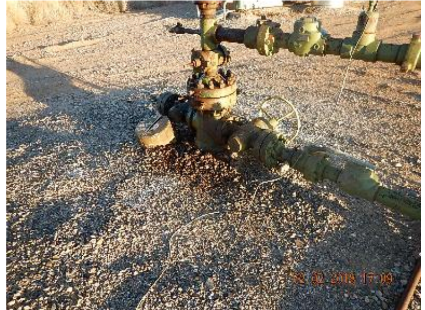
Photo 4: Impacted soil and gravel at wellhead.
