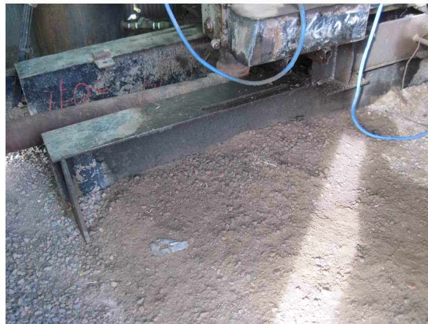
SOILED DIRT INSIDE MOTOR MOUNTS
