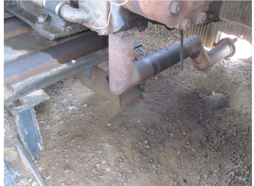
SOILED DIRT INSIDE MOTOR MOUNTS
