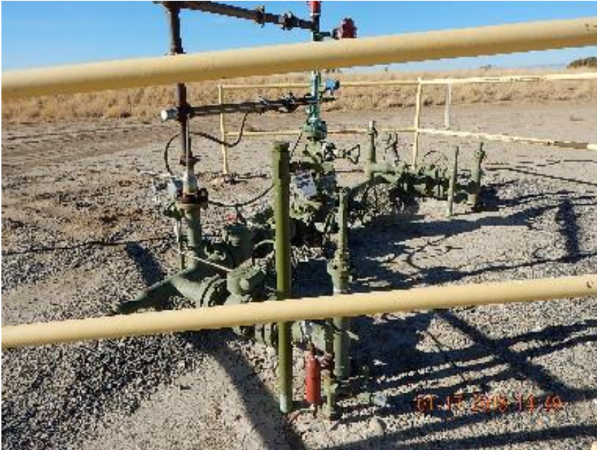
Photo 3: Unused riser at wellhead.
