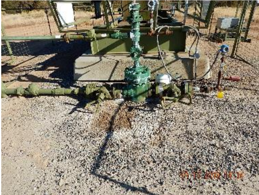
Photo 5: Impacted soil at wellhead.
