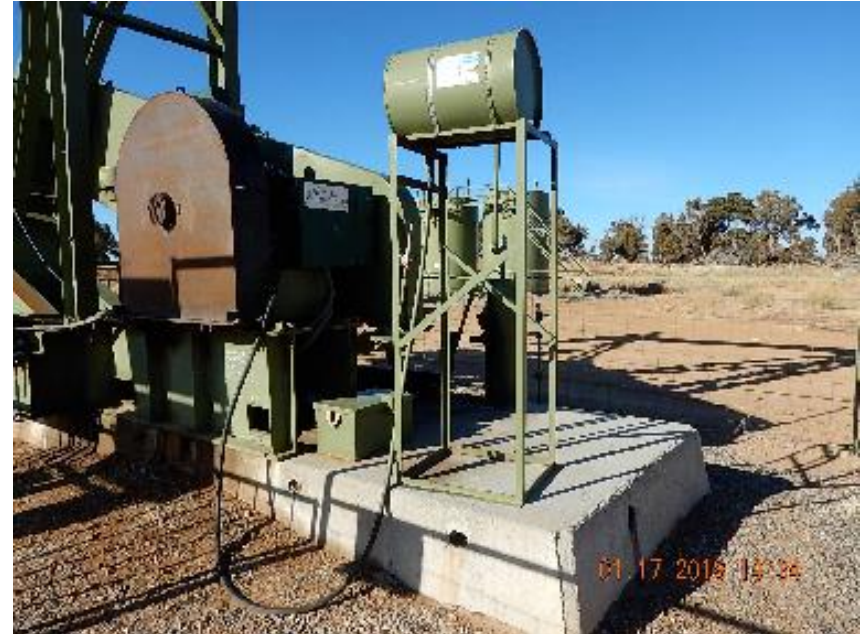
Photo 6: Lube oil tank without spill prevention.
