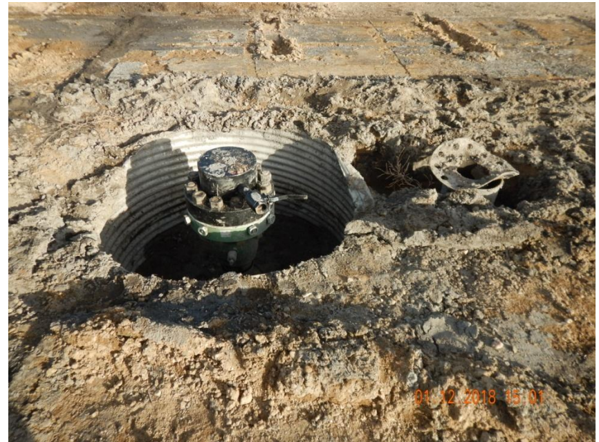
Photo 2. Photo taken from an adjacent wellhead at location. Photo illustrates the rat hole was partially covered up.
