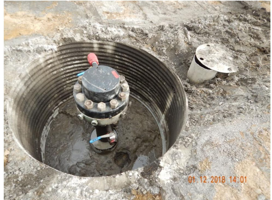
Photo 2. Photo taken from an adjacent wellhead at location. Photo illustrates the rat hole was covered up.
