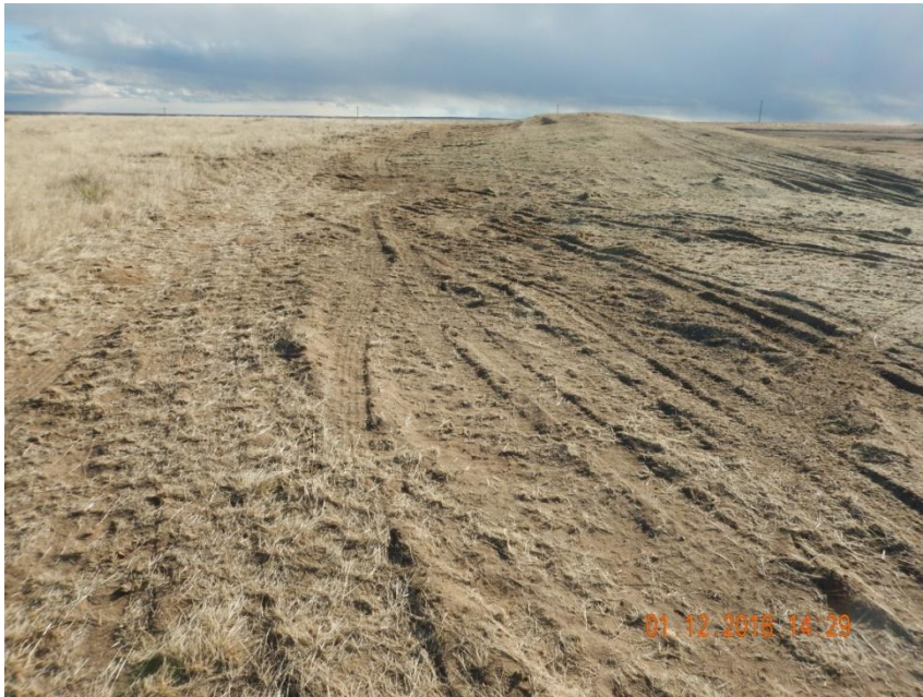
Photo 13. Photo taken from the northeast perimeter of the location, facing South. Operator does not have sufficient stormwater BMPs along the perimeter of the location.
