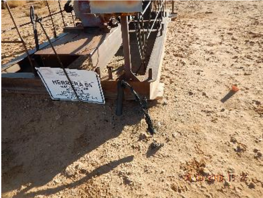
Photo 15: Disconnected power line at wellhead.
