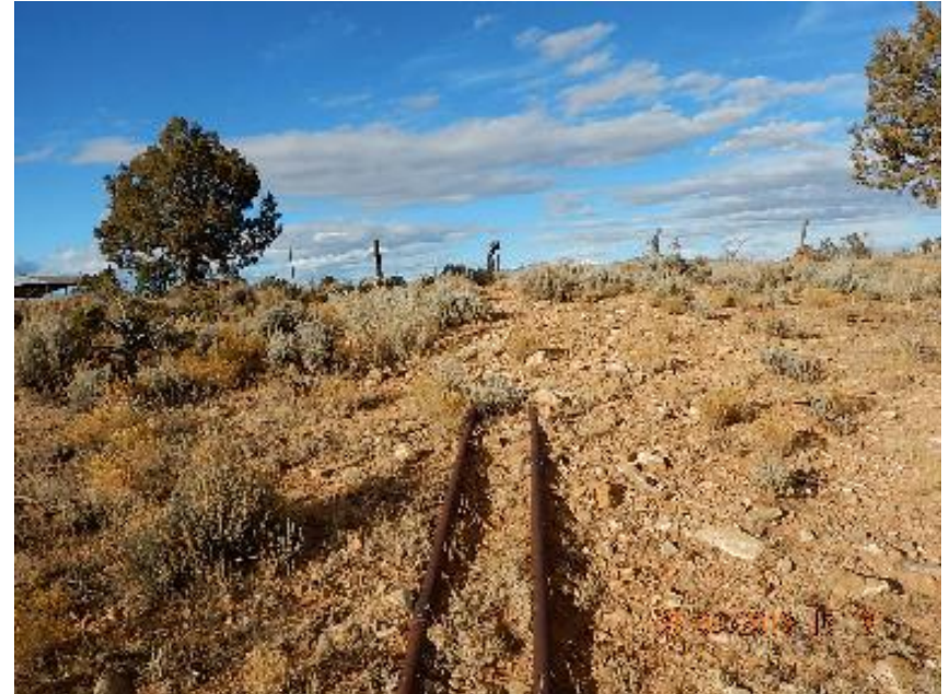
Photo 6: 3" steel lines on edge of slope with pump jack in background.
