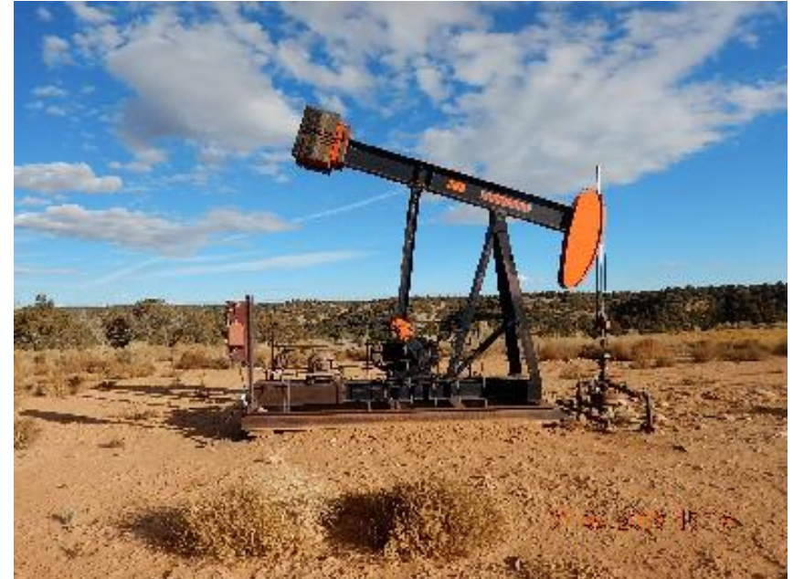
Photo 2: Pump jack, electric panel, and wellhead..
