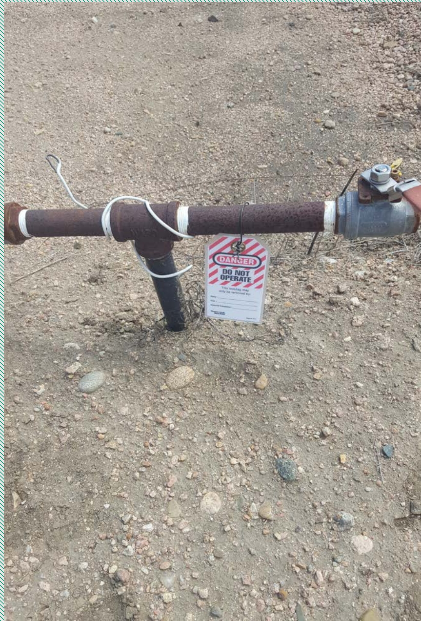
Figure #2 Unused risers have labeled
