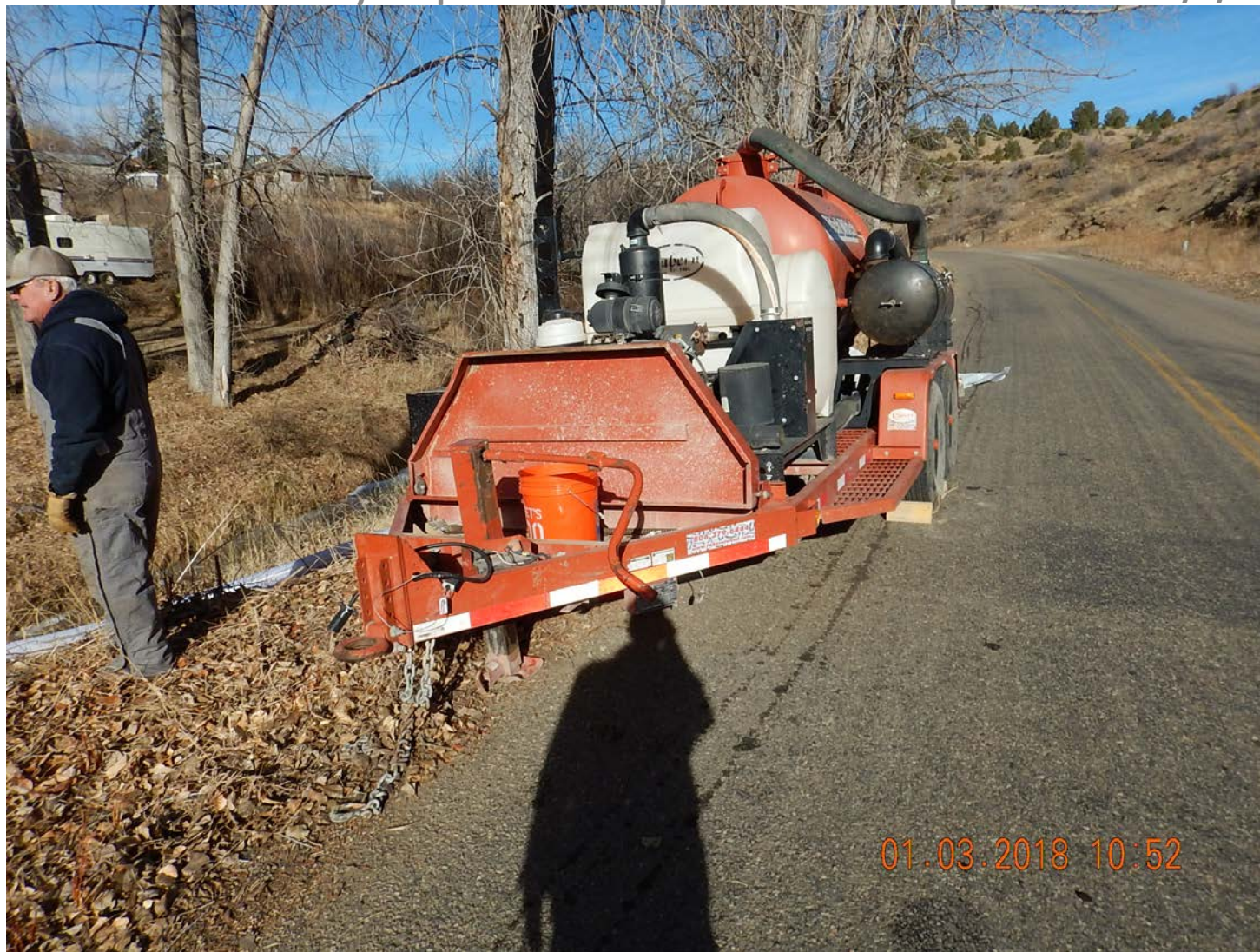
Vacuum trailer stationed at the base of Wet Canyon and was actively pumping impacted water from Wet Canyon. Located at COGCC Sample #1 location.
