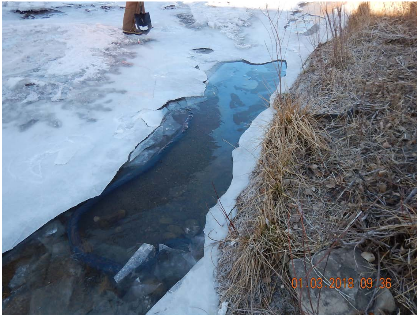
COGCC Sample #2. Surface water sample obtained from the Purgatorie River here. This location is where Wet Canyon flows into the Purgatorie. Saturated boom and thin oil sheen visible. Coordinates 37.131893, -104.847150
