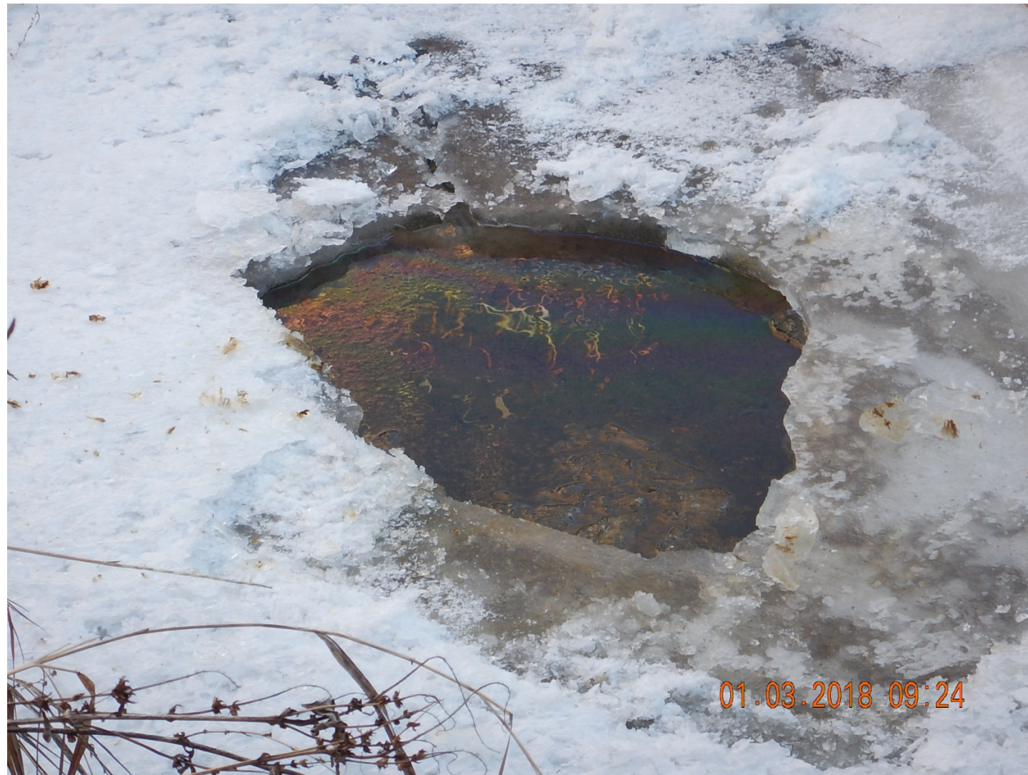
COGCC Sample #1. Surface water sample obtained from Wet Canyon here. Coordinates 37.13234, -104.84719. Very thin oil sheen observed.
