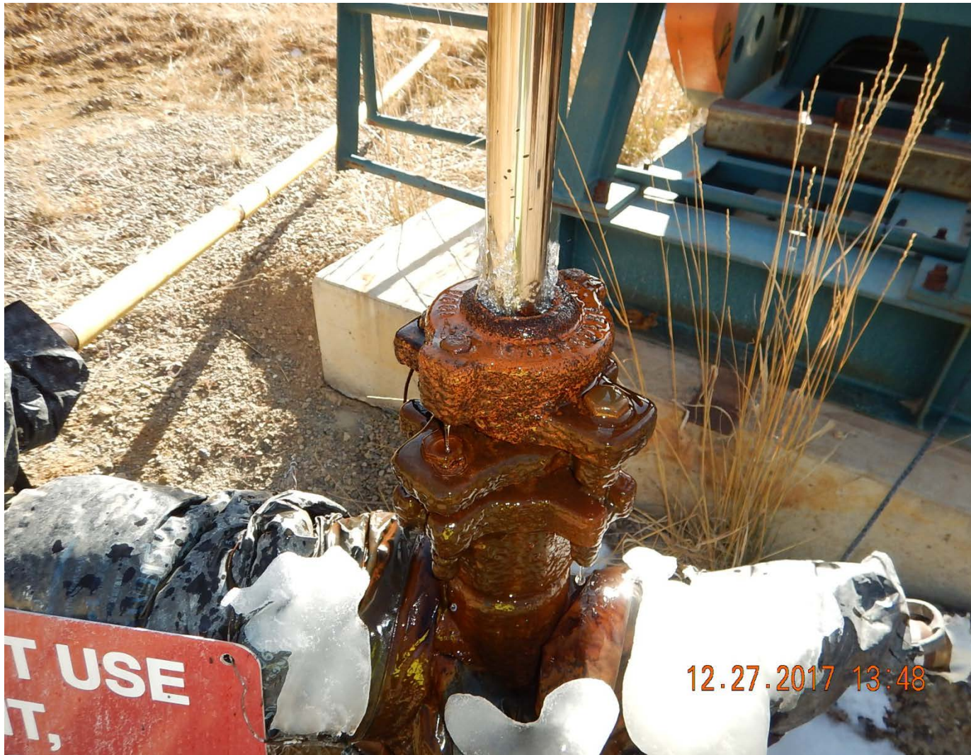
Small leak from wellhead observed. Produced water from leak froze around wellhead.
