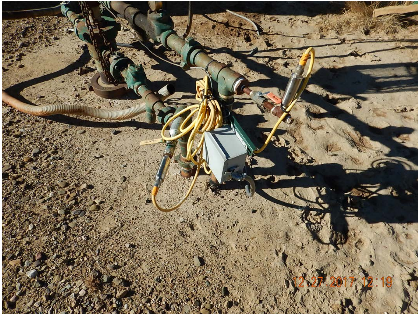
Wellhead equipped with two transducers.
