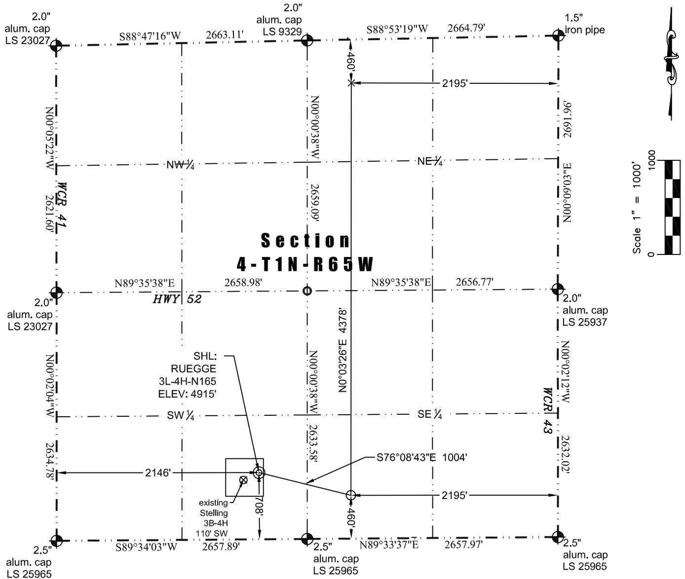
In accordance with a request from Jay Knutson of Crestone Peak Resources, Washburn Land Surveying, LLC has determined the location of the **RUEGGE 3L-4H-N165** well site to be SHL: 708' FSL and 2146' FWL, (TPZ: 460' FSL and 2195' FEL), (BHL: 460' FNL and 2195' FEL), as measured at ninety (90) degrees from the section lines of Section 4, Township 1 North, Range 65 West of the 6th Principal Meridian, Weld County Colorado.
