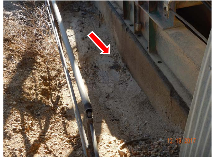
Photo #4 – Localized accumulation of lube oil underlying northeast side of pump jack after oily waste had been removed by operator in response to previous FIRs.
