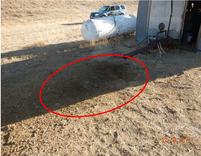
Photo #5 - Localized accumulation of blow-through motor oil underlying muffler at NW end of pump jack after oily waste had been removed by operator in response to previous FIRs.
