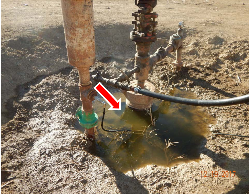
Photo #3 – Pool of water remaining at wellhead has been documented in field inspection reports dating back to June 22, 2017. Periodic bubbling of gas from area beneath wellhead was observed on date of inspection.
