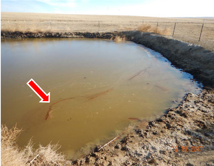
Photo #23 – Trace amount ( <<1\% ) of free-phase hydrocarbons remained on produced water pit on inspection date.
