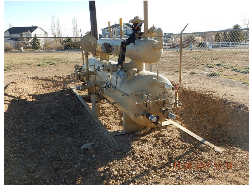
Horizontal separator – Unused equipment
