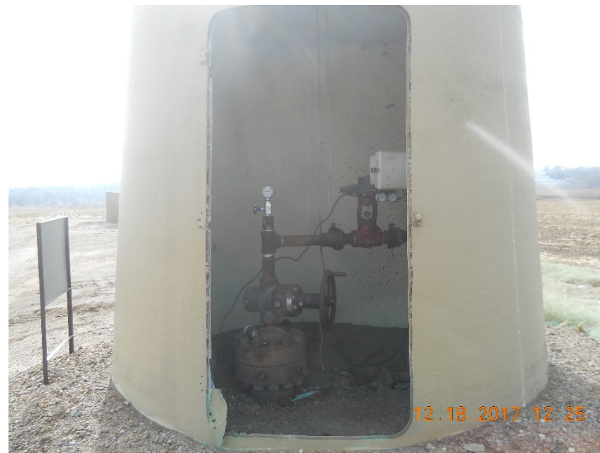
Wellhead looking south, fiberglass enclosure around wellhead
