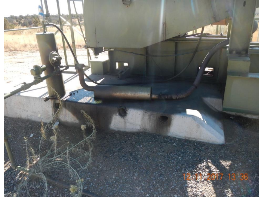
Stained concrete pad and surrounding area near muffler exhaust.
