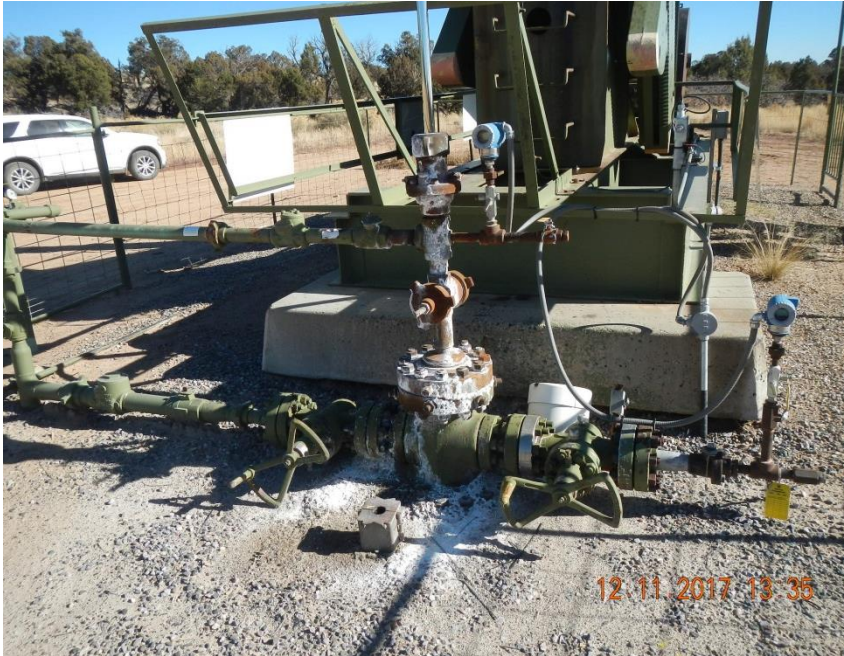
Well head and surrounding area stained with white residue.
