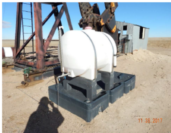
Photo #4 – Day tank at SE corner of pump jack has adequate secondary containment device.
