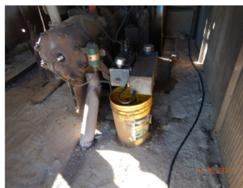
Photo #9 - Historical accumulation of oil-stained soil beneath prime mover (1).
