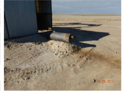
Photo #8 – Localized accumulation of oil-stained soil at prime mover exhaust.
