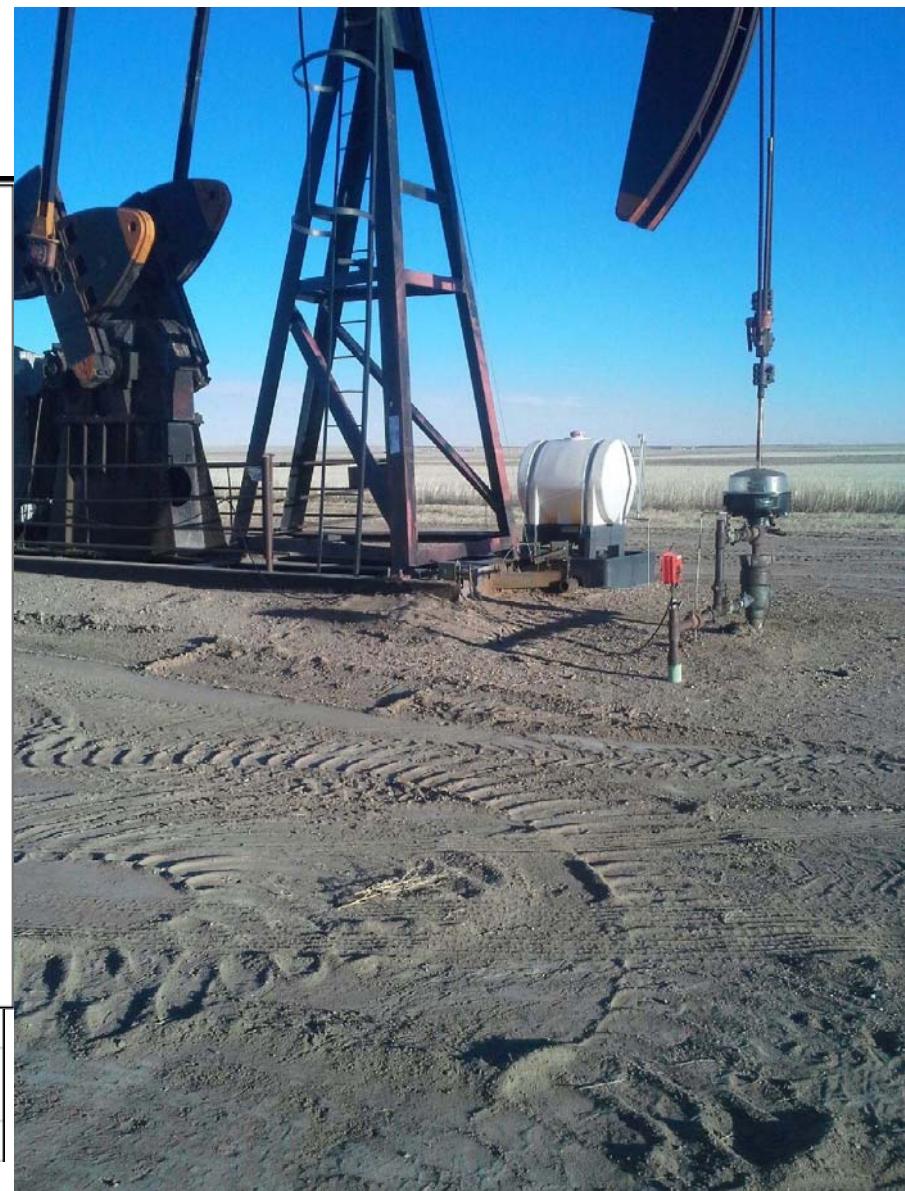
Photo #4 – Day tank at SE corner of pump jack has adequate secondary containment device.
