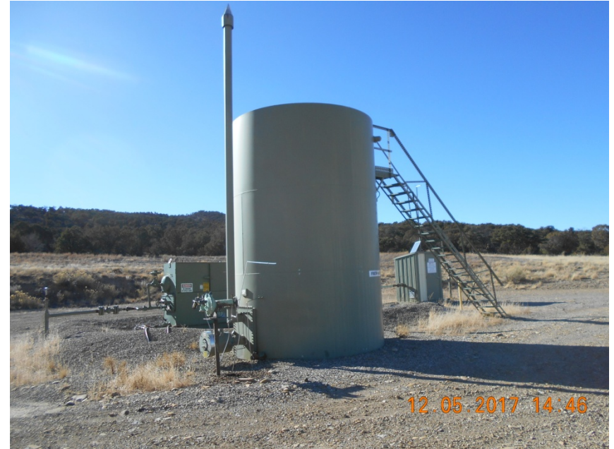
Heated freshwater tank
