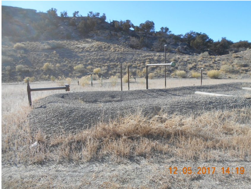
Unused/unmarked risers on SW corner of pad.
