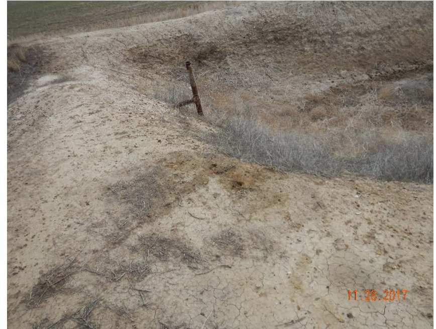
Photo #30 – Oil-stained soil and pipe riser at NE section of south produced water pit.
