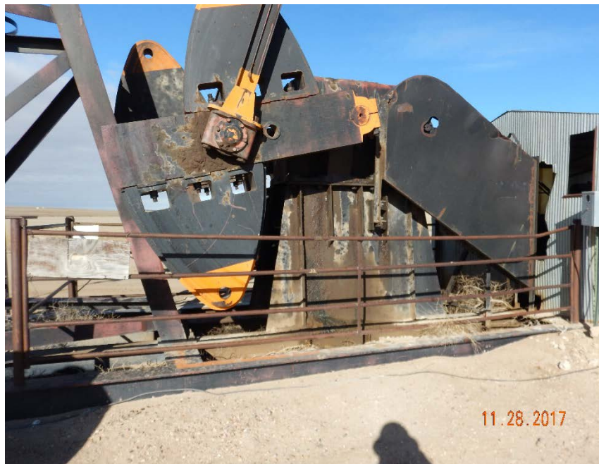
Photo #5 – Oil-stains on east side of pump jack.
