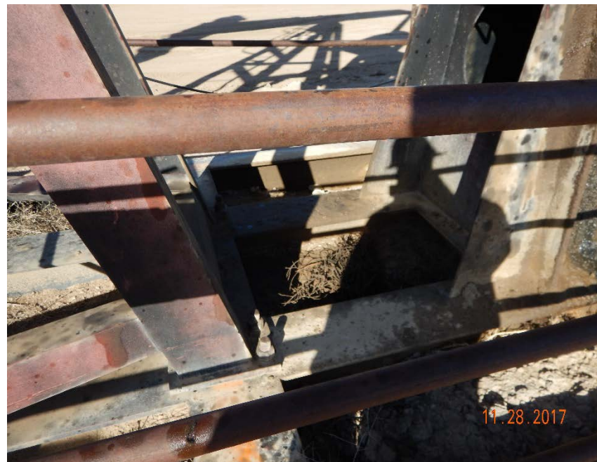
Photo #6 – Oil-stained soil and weeds accumulating beneath pump jack.
