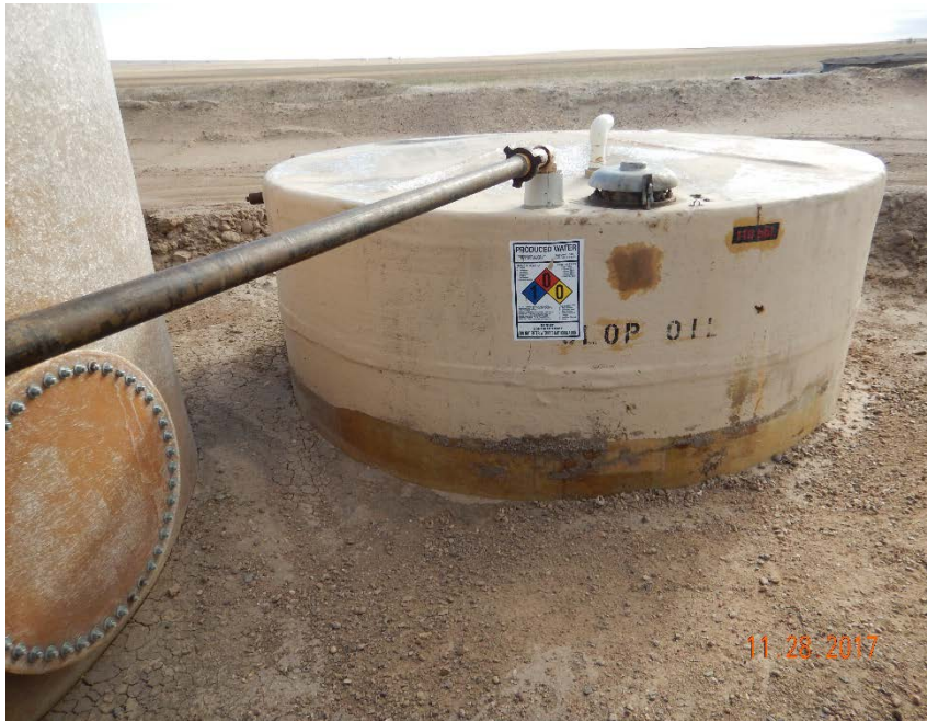
Photo #21 – 110 bbl fiberglass produced water PBV.
