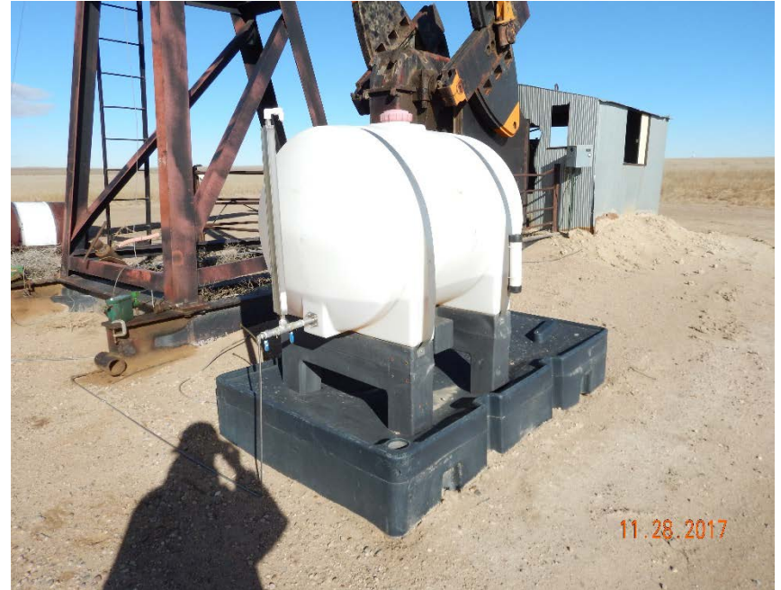
Photo #4 – Day tank at SE corner of pump jack has adequate secondary containment device.
