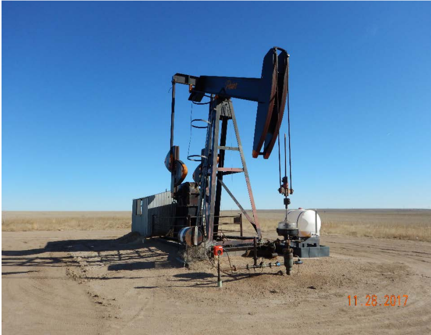
Photo #1 – View of wellhead and pump jack from SW corner. Note accumulation of wind-blown weeds and absence of secondary containment device beneath day tank at SW corner of pump jack.
