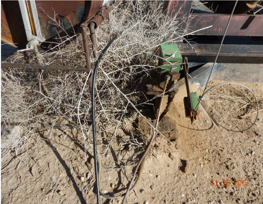
Photo #3 – Localized accumulation of oil-stained soil and wind-blown weeds beneath day tank and SW corner of pump jack.
