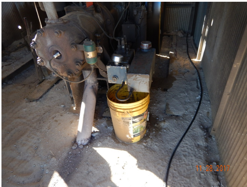
Photo #9 – Historical accumulation of oil-stained soil beneath prime mover (1).
