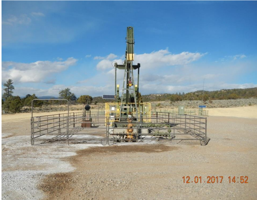
Merry Federal #2 well head, pump jack, and stained soil.
