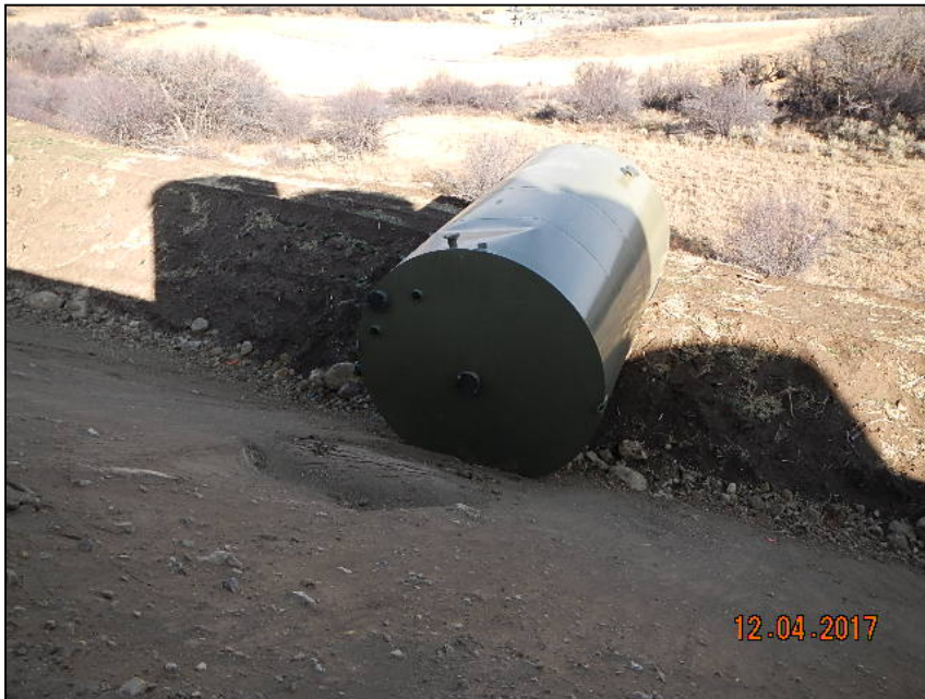
Photo 3. Production tank off location in Stormwater ditch on North side of location.
