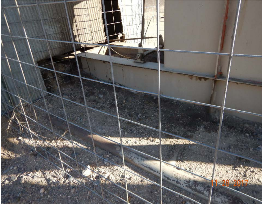
Photo #5 – Oil-stained soil beneath NW corner of pump jack.
