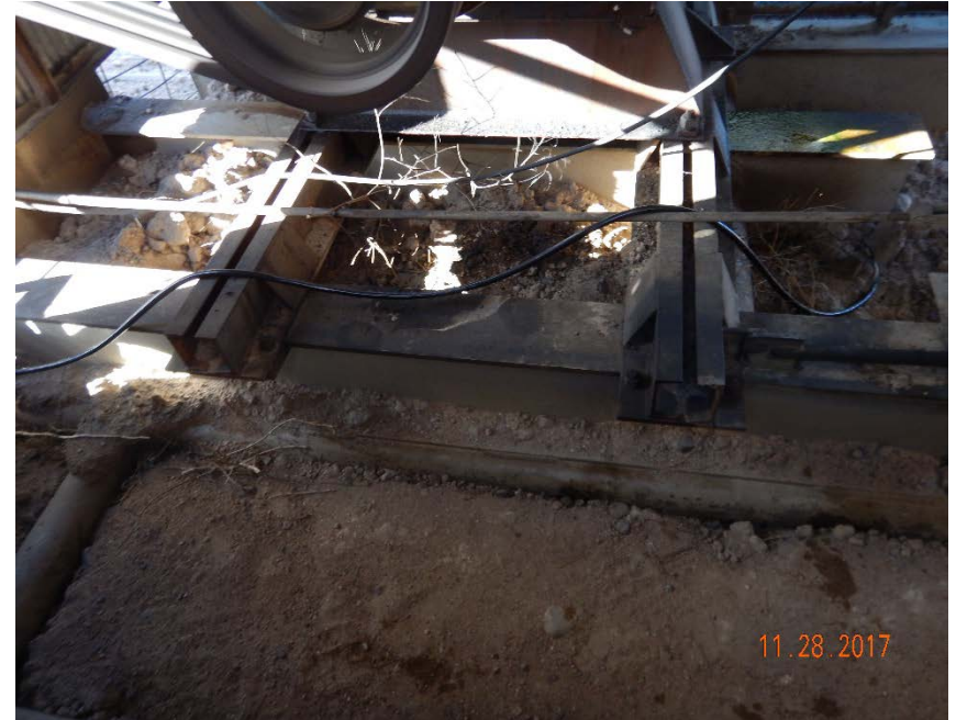
Photo #6 – Oil-stained soil beneath prime mover (1).
