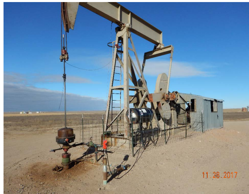
Photo #2 – View of wellhead, looking northwest. Note localized, oil-stained soil at wellhead and day tank at SE corner of pump jack lacking secondary containment device.
