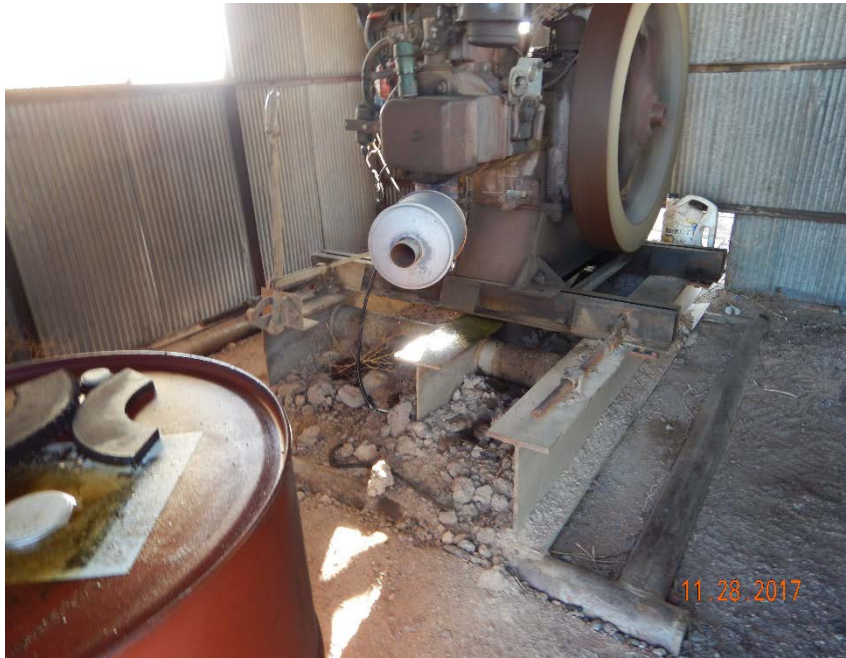
Photo #7 – Oil-stained soil beneath prime mover (2).
