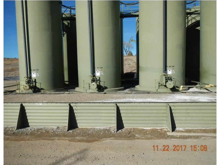
Damp soil outside of secondary containment ring.
