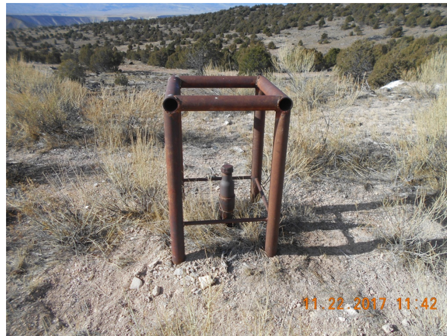
Capped risers with pipe barricade.
