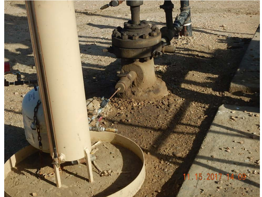
Photo 2: Stained soil at wellhead. Bradenhead plumbed to surface
