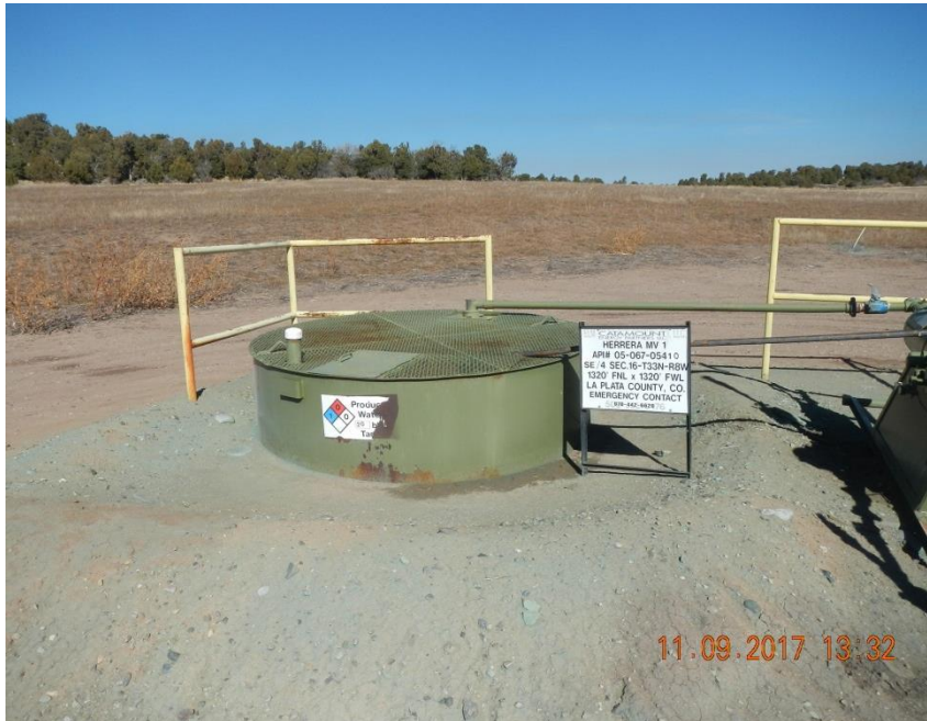
Open topped produced water vessel with expanded metal cover.
