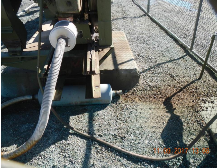
Stained soil and gravel near muffler exhaust.
