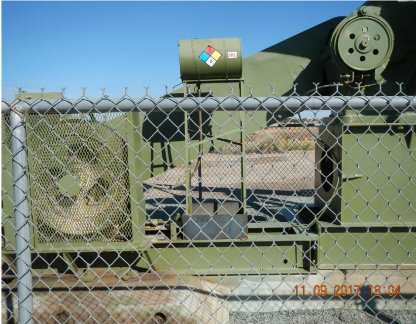
Secondary containment for lube oil container.
