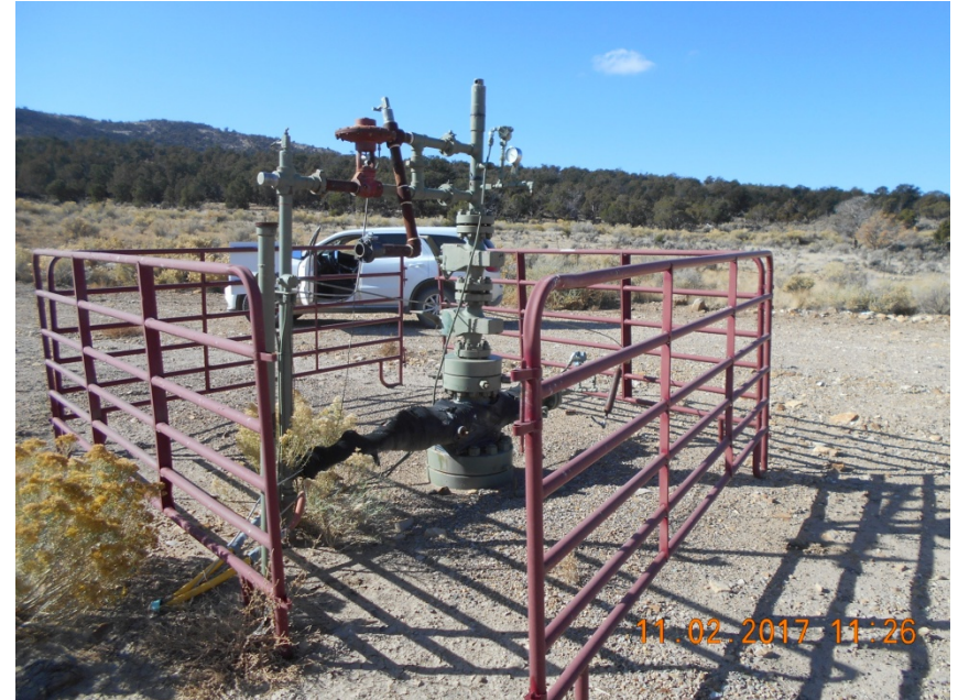
Wellhead with unused risers.
