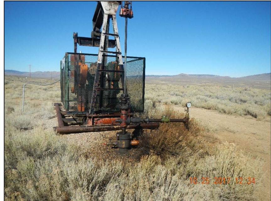
Photo 2. Stained soil at wellhead.
