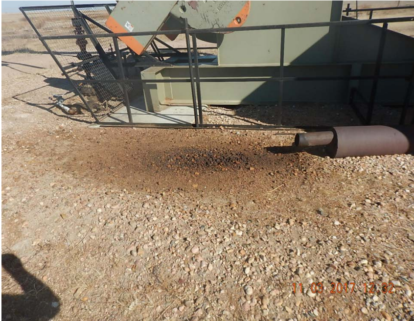
Photo 7: Stained soil at exhaust
