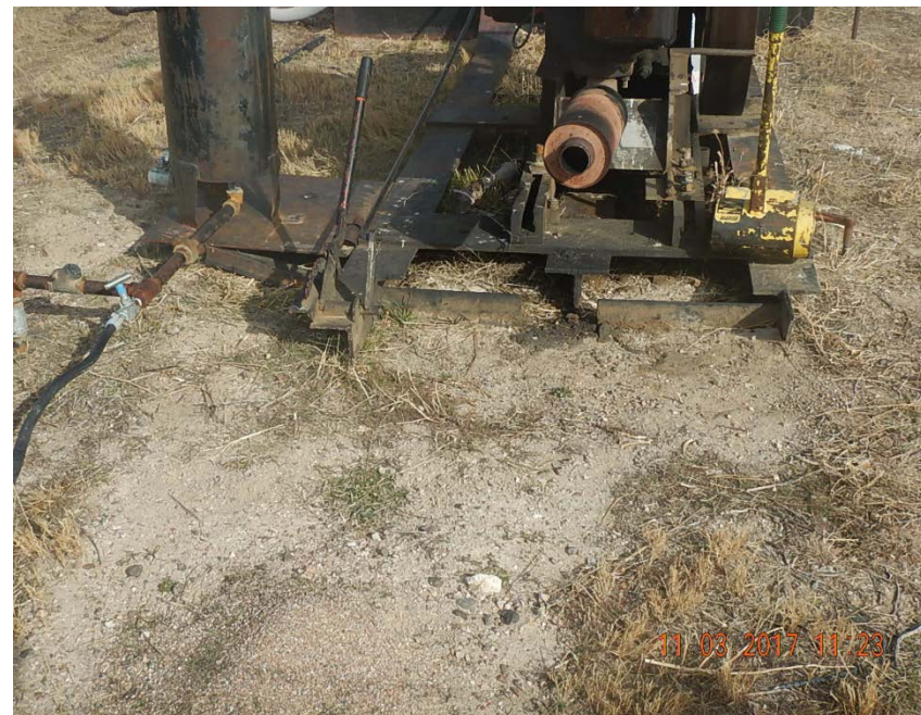
Photo 4: Stained soil at engine
