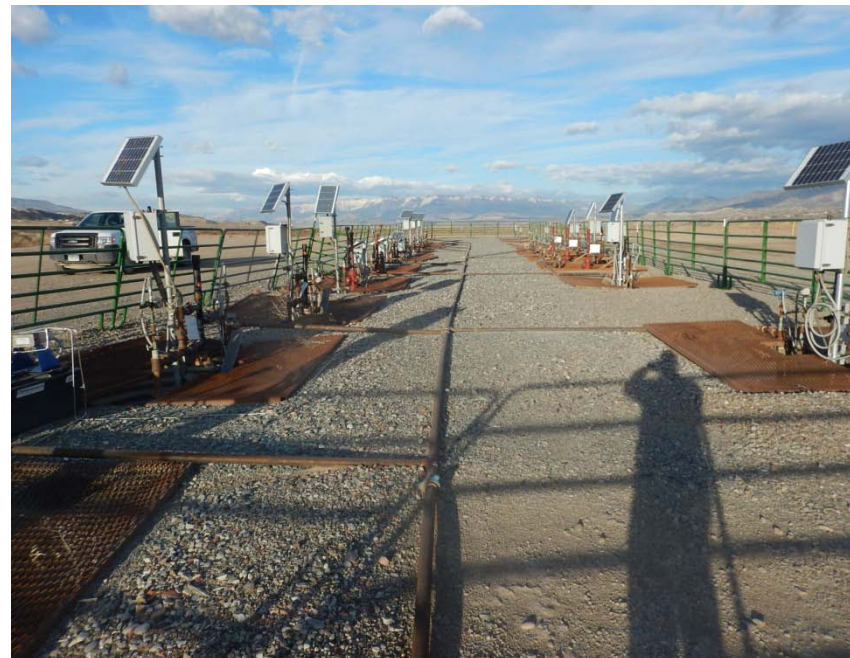
Wellheads with 2" pipe manifold connecting Bradenheads
