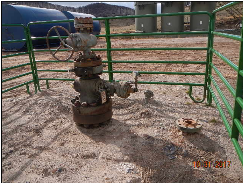
Photo 1. Well has been disconnected.
