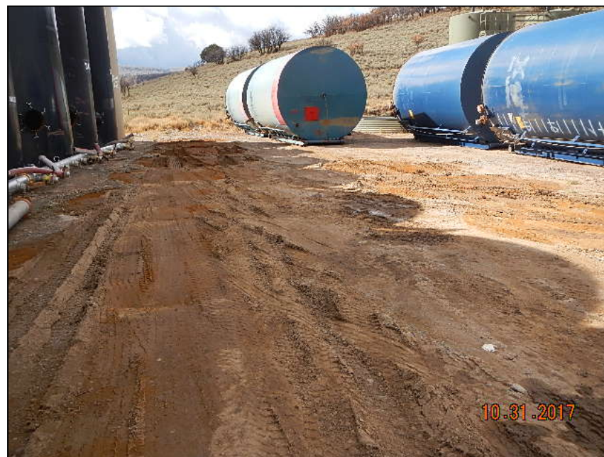
Photo 4. Staining around and under unused tanks.
