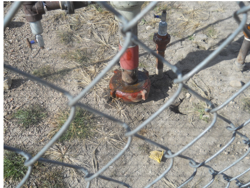
Stained soil around wellhead needs to be cleaned up. Appears that wellhead packing is leaking or has leaked at some point
