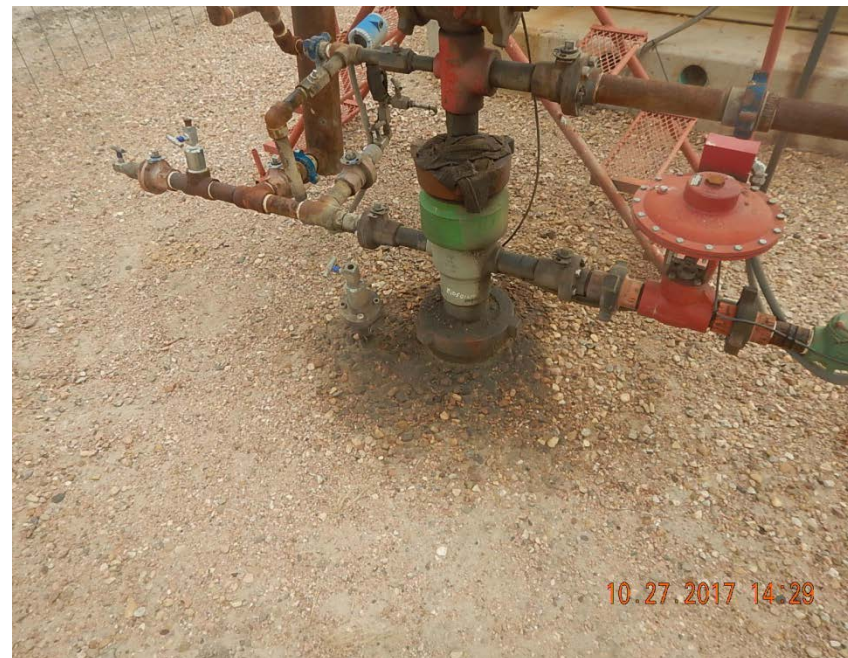
Photo 2: Stained soil at wellhead
