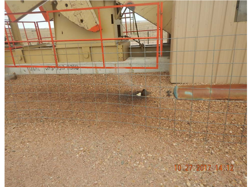
Photo 2: Stained soil at exhaust
