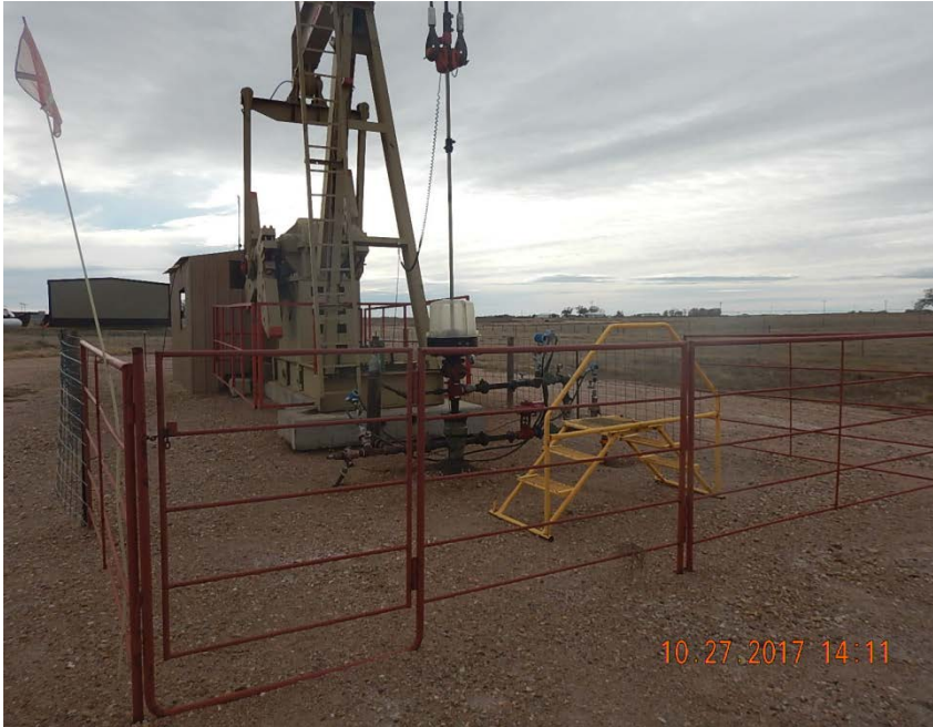
Photo 1: Wellhead, looking SW. Stained soil at wellhead.
