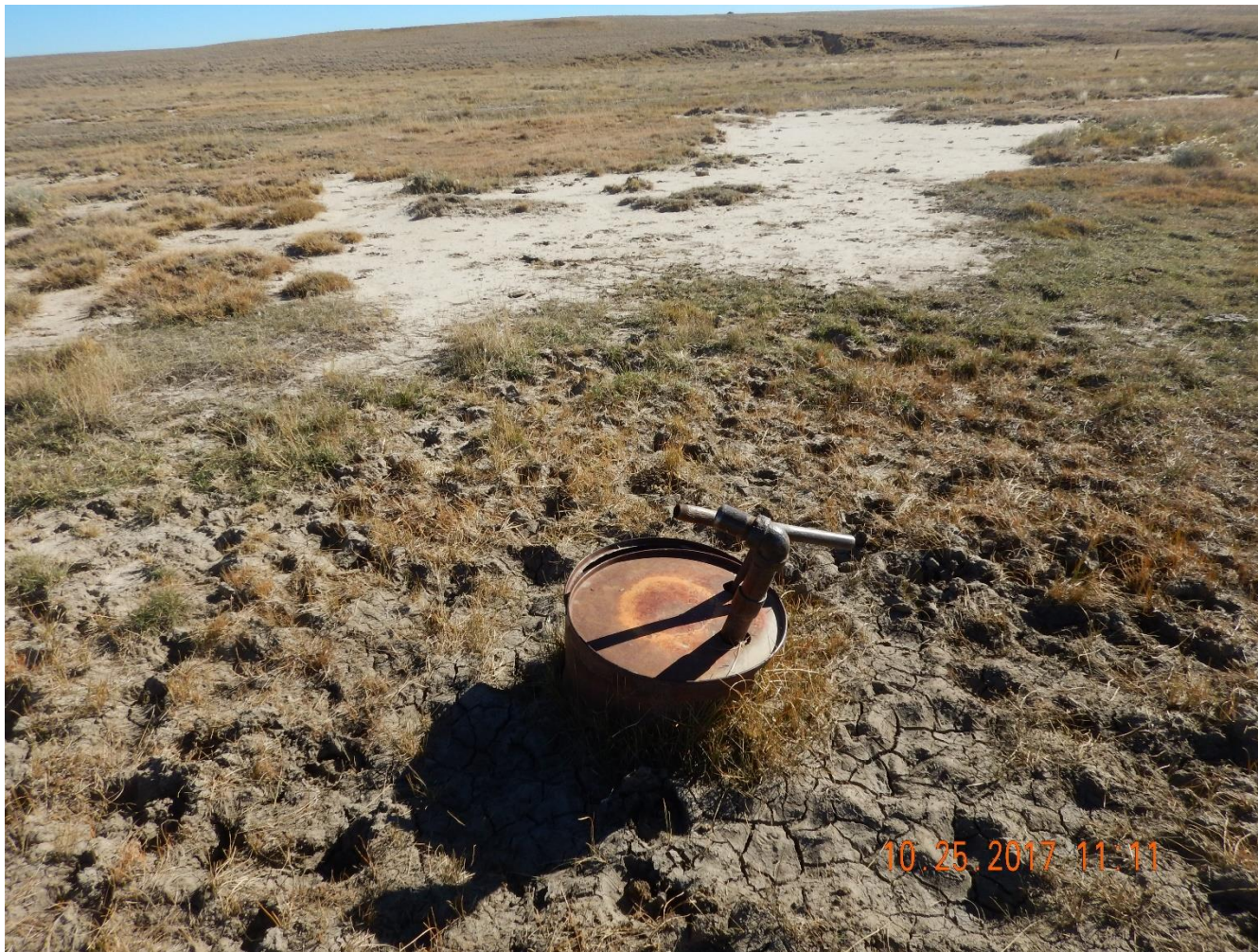
Photo 1: Photo taken from the location, facing east. Previous inspection indicate that the "valve body/bodies buried in barrel and well not capped off or buried". Photo shows equipment remains on the location.
