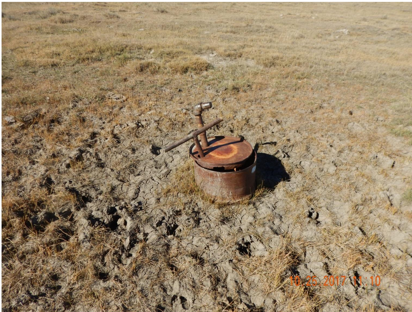
Photo 2: Photo shows pipe and valve in barrel. The barrel was partially filled with what appeared to be water.
