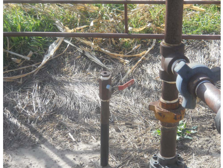
1" unused/unmarked steel riser at wellhead
