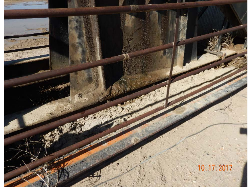
Photo #4 – Recent lube oil stains on east side of pump jack.
