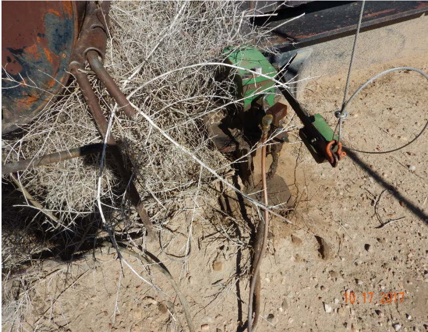
Photo #7 – Localized accumulation of oil-stained soil and wind-blown weeds at SW corner of pump jack.
