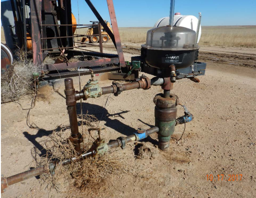
Photo #3 – Localized accumulations of oil-stained soil and wind-blown weeds at wellhead. Note fresh crude oil stains on equipment.
