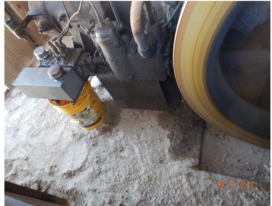
Photo #6 – Localized accumulations of oil-stained soil beneath prime mover.
