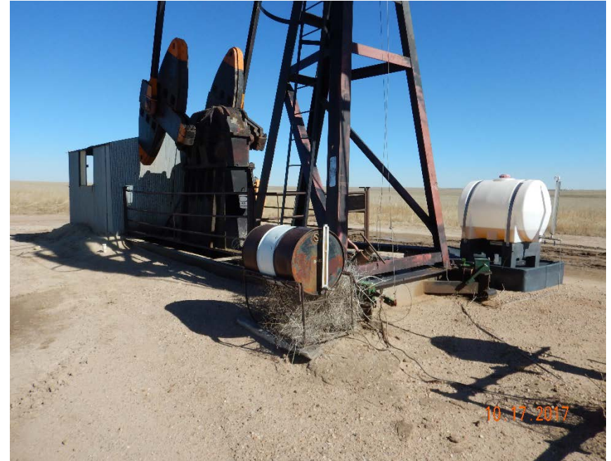
Photo #2 – Day tanks at south end of pump jack. 55-gallon drum/day tank lacks secondary containment device and exhibits historical accumulation of both impacted soil and wind-blown weeds underneath.
