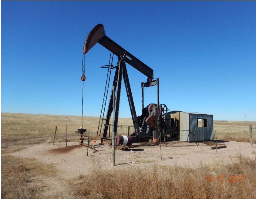
Photo #1 – View of pump jack and wellhead from SE corner. Note oil-stained soil beneath wellhead and shed.
