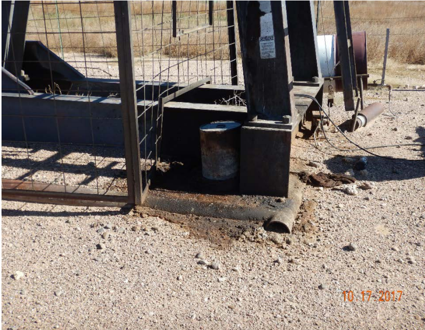
Photo #3 – Localized oil-stained soil beneath 1-gallon chemical storage container (which lacks secondary containment device) at SW corner of pump jack.
