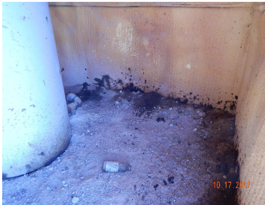
Photo #21 - Oil-stained soil and historical accumulations of oily waste inside of separator shed (2).
