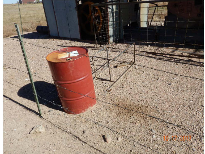
Photo #4 – 55-gallon drum on west side of pump jack is open to atmosphere and lacking secondary containment device. Drum contained unknown amount of fluid on date of inspection.
