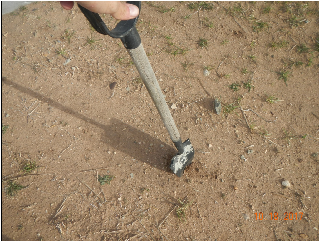
Photo 12. There are areas where the soils appear to be compacted. The shovel is unable to penetrate the soil surface.
