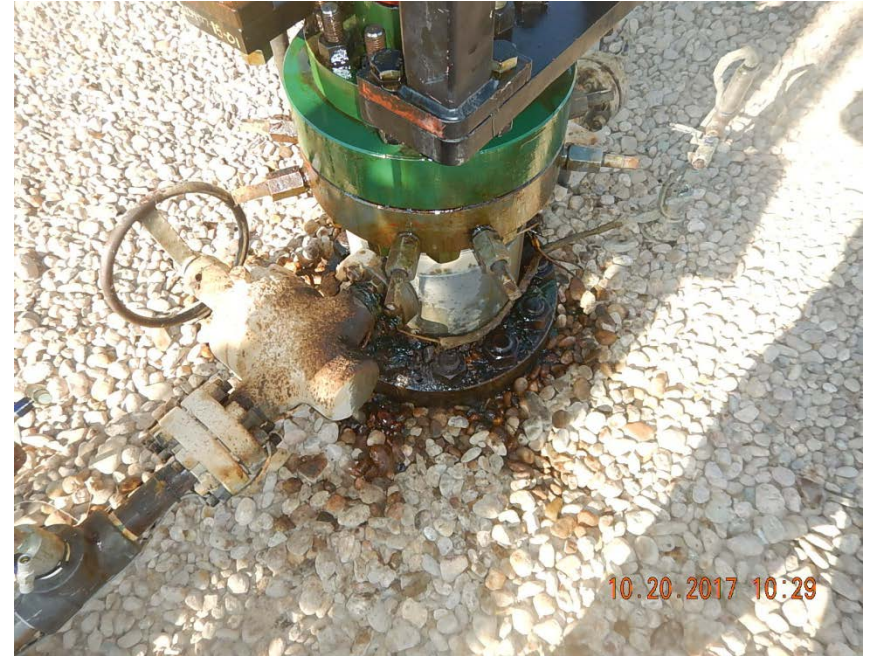
Photo 4: Stained soil at wellhead
