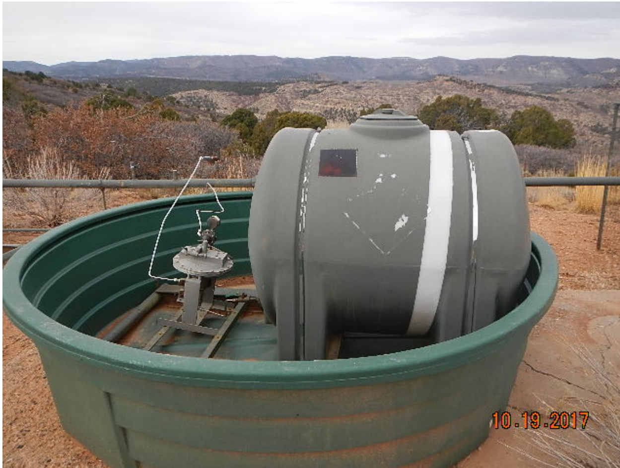
Photo 1. Signs on Methanol tank are not legible..
